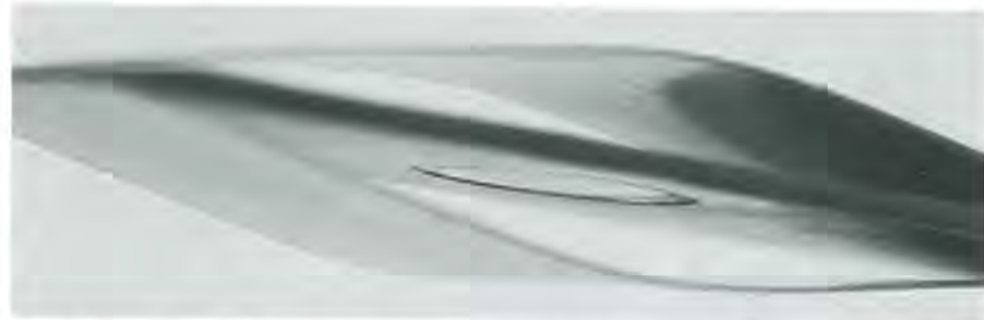
Figure 5. Two differential (back to back) noncontact sensors mounted in a 1.5 mm thick assembly are looking at the underside of two thin leaf springs that in turn contact a gap space with a range of 1.5–5.0 mm. Since there are two opposed spring forces, the wand assembly self-centers itself in the gap, almost doubling the measurement range of previous configurations.
